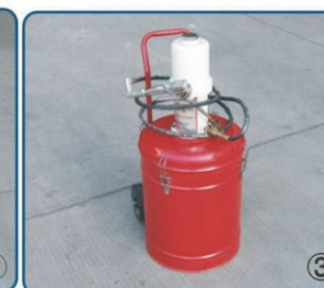
3 - Close the oil dispenser cover and shut it with the clamps
