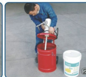
2 - Open the oil dispenser cover and put the barrel inside
