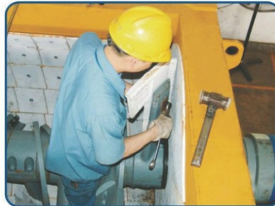
Side Mixing Blade adjustment
