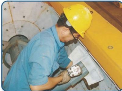
Central Mixing Blade adjustment
